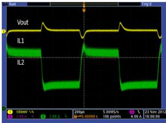
Figure 37. Load Transient, Current Share Mode Operation ( I_O = 4\text{ A} - 9\text{ A} )
