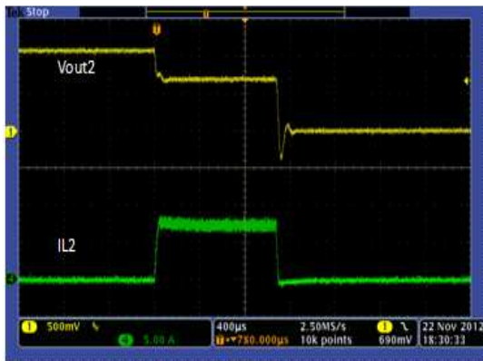
Figure 29. Over Current Protection, Buck 2
