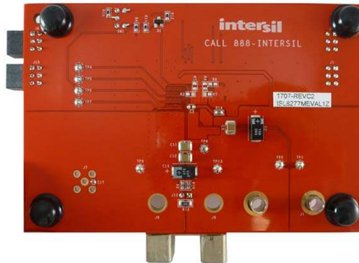
Figure 3. ISL8277MEVAL1Z Evaluation Board (Bottom Side)
