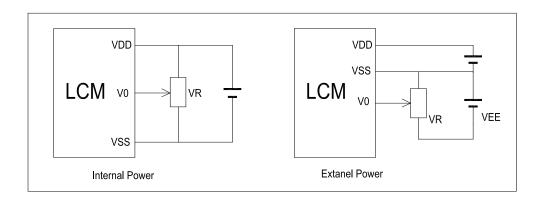
$V_{\text{DD}^{\sim}}V_0\text{: LCD}$  Driving voltage
