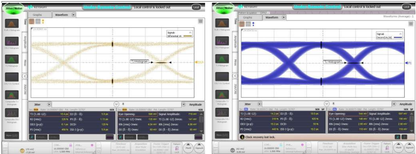
Figure 7. SN75LVPE4410 Typical Jitter Characteristics in TI Evaluation Board. Left - Input to the Device, Right - Output of the Device with Jitter Decomposition Shown.
