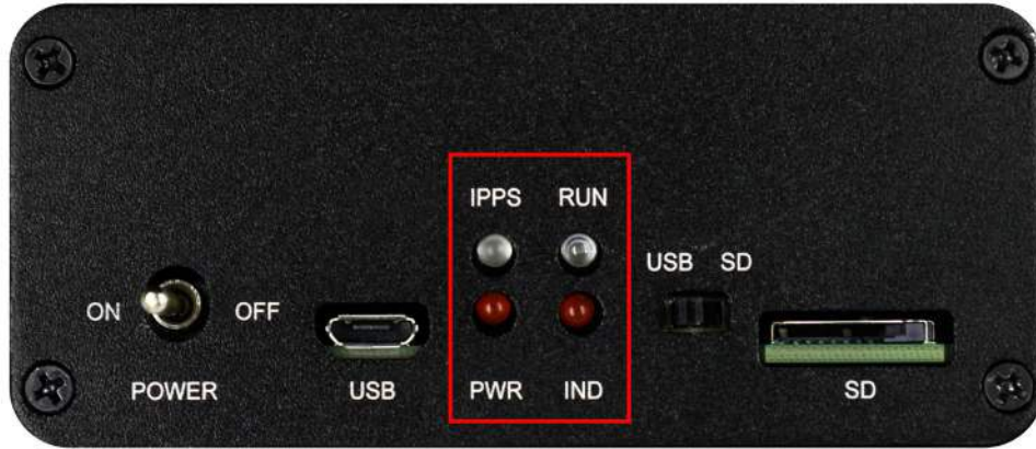
Figure 8: Operation Status Indication LEDs
