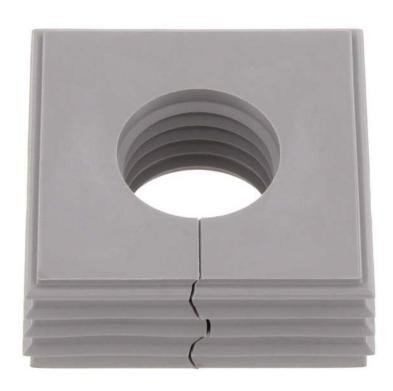
Seal, Mounting type: Plug in, Length x width: 42.8 mm, Max. cable diameter: 21 mm, IP 66, Colour: Grey
