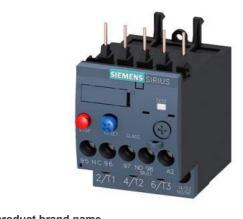
Overload relay 7.0...10 A Thermal For motor protection Size S00, Class 10 Contactor mounting Main circuit: Screw Auxiliary circuit: Screw Manual-Automatic-Reset
