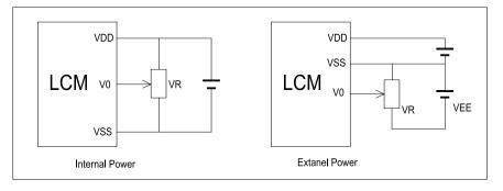
VDD~V0: LCD Driving voltage VR: 10k~20k
