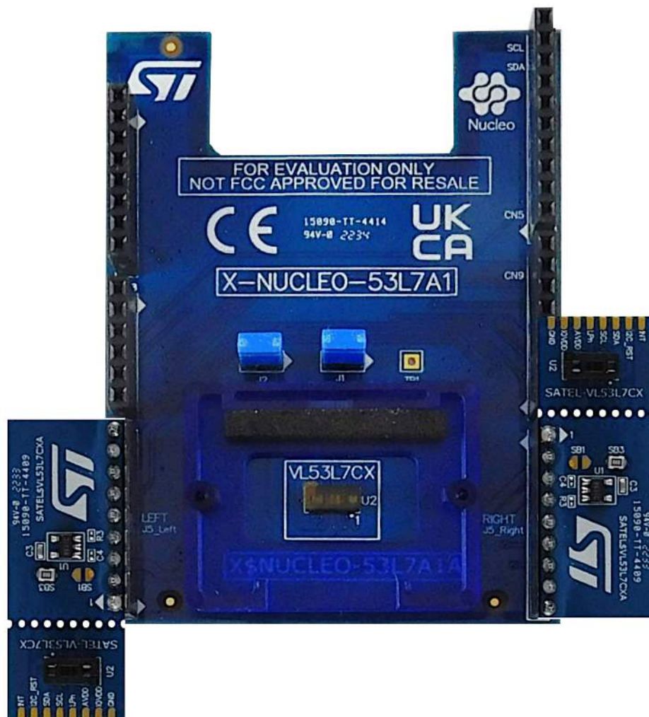
Figure 2. SATEL-VL53L7CX breakout boards connected to the X-NUCLEO-53L7A1 expansion board
