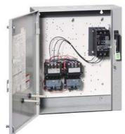
2-speed 3-phase motor starter Size 1 Two separate windings Constant or variable torque Solid-state overload relays Low SPD OLR range 3-12A High SPD OLR range 3-12A 110V 50HZ / 120V 60HZ coil Combination type 10Amp circuit breaker Enclosure NEMA type 4/12 Water/dust tight for outdoors
