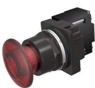
30mm BlackMax, Epoxy Coated Corrosion Resistant Complete Metal Unit Illuminated Push-Pull Operator Transformer type, 600V AC LED Lamp Mushroom Head Cap Small 1 3/4" (44.5 mm) Plastic, Red 2 Position Maintained, Pull-to-Release UL Listed, CSA Certified NEMA 1,3,3R,4,4X,12,13 & Automotive Standards
