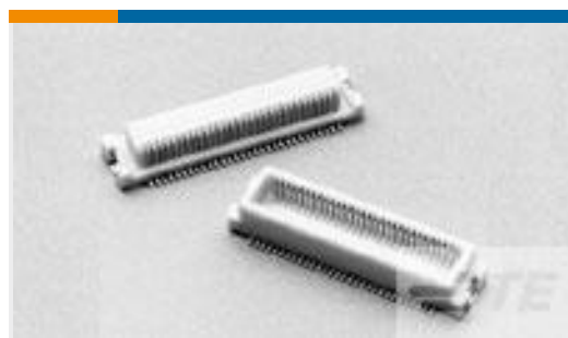
TE Part #1-1827876-0 Header Assembly: Wire-to-Board, 5A, gold or tin plated
