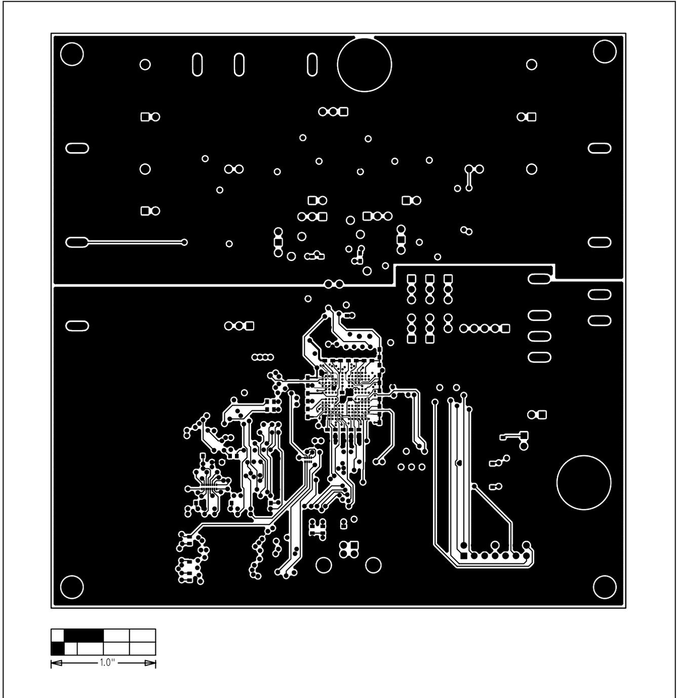
Figure 9. MAX1379 EV Kit PCB Layout—Solder Side
