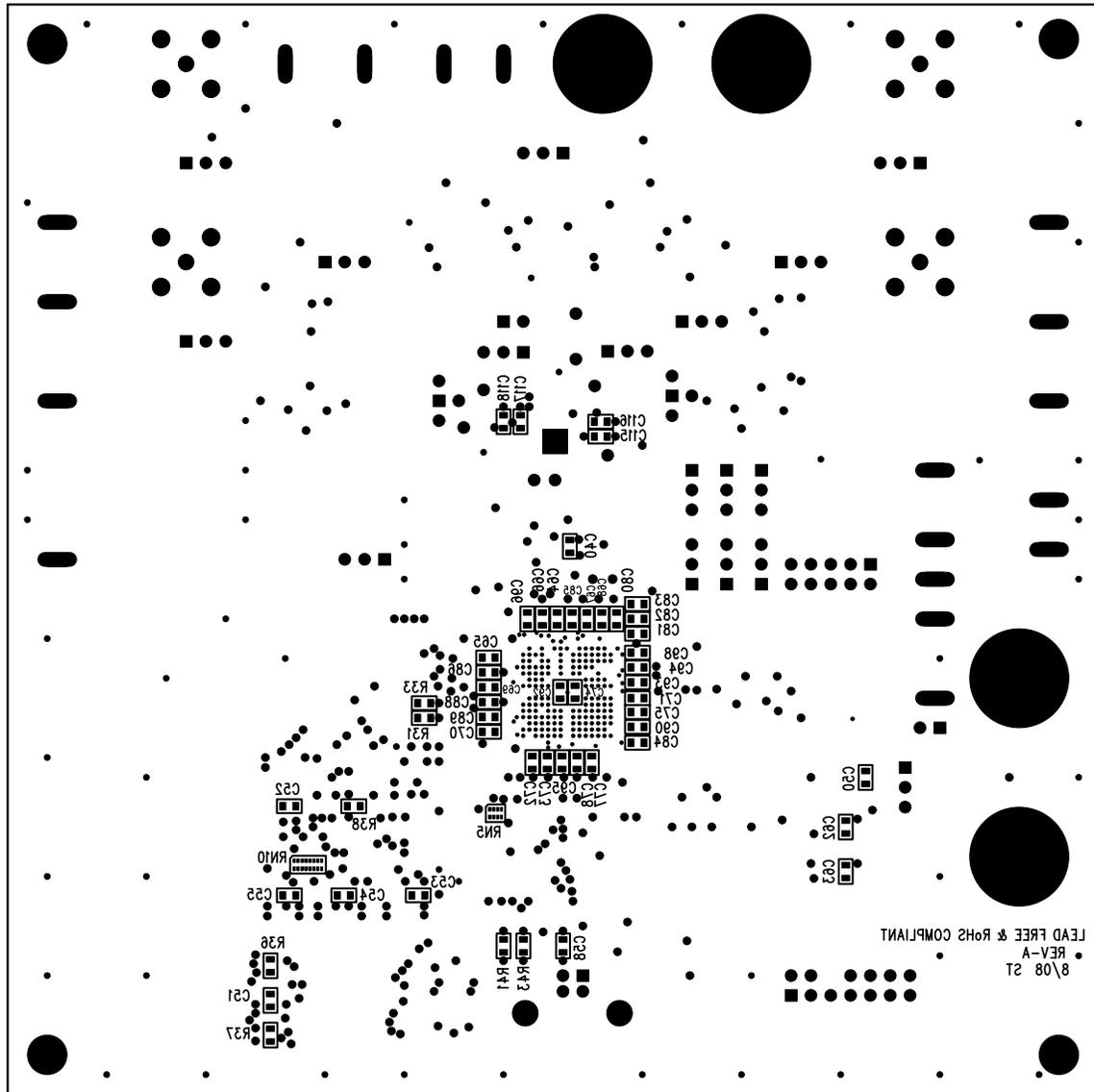
Figure 10. MAX1379 EV Kit Component Placement Guide—Bottom Silkscreen
