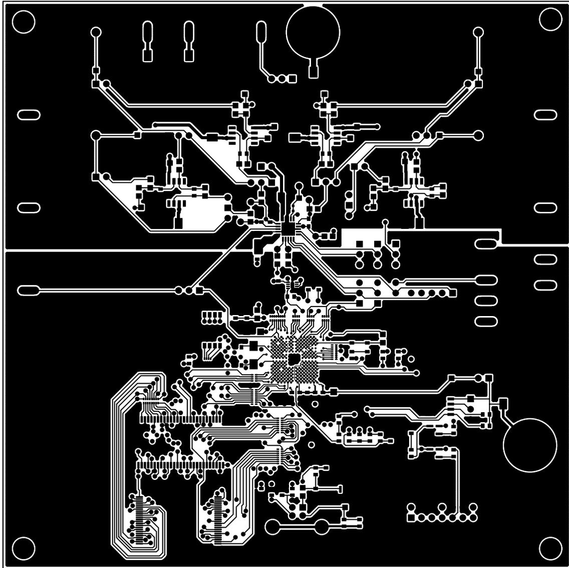
Figure 4. MAX1379 EV Kit PCB Layout—Component Side
