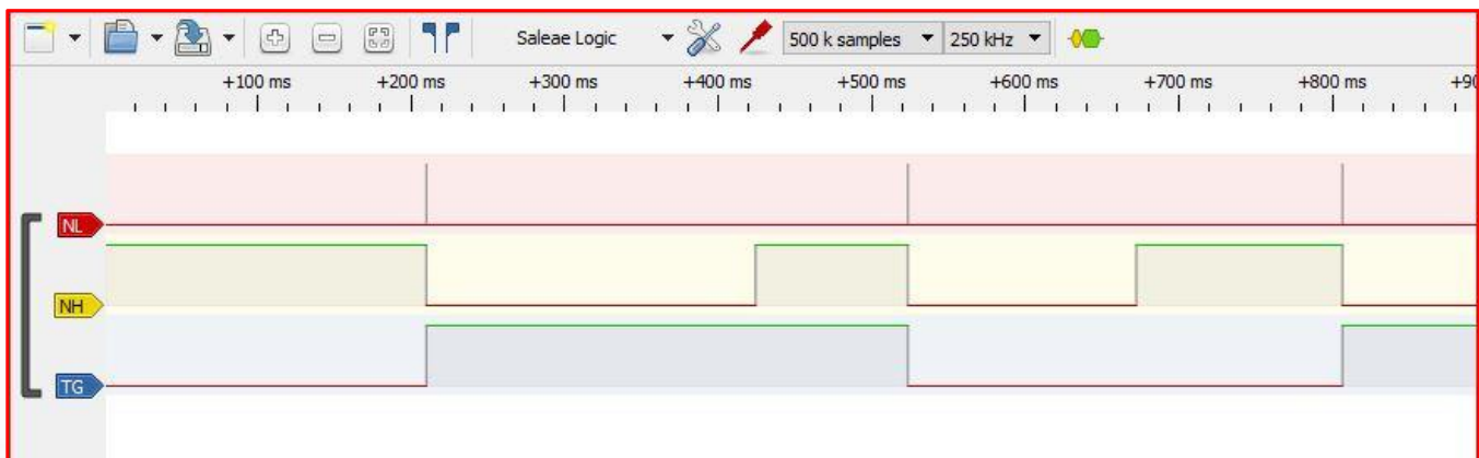
NL Output Acknowledged by Host with Handshake
