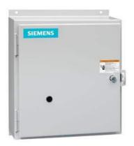
Reversing contactor Size 2 1/2 Three phase full voltage Contactor amp rating 60Amp 3 w 110-120/220-240VAC 60HZ coil Non-combination type Enclosure NEMA type 12 Dust/drip proof for indoors Standard width enclosure
