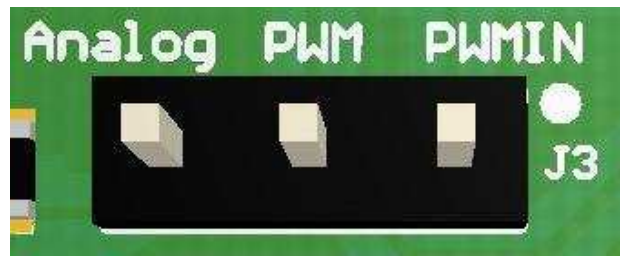
Figure 11. Speed Command Input Select Header (J3)
