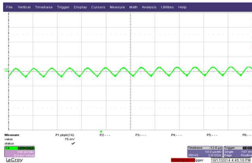
Figure 6. Output Ripple and Noise (230 V/60 Hz, load = 65 W)
