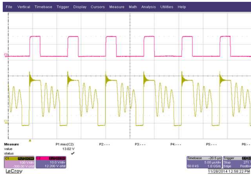
Figure 13. C1 = V_{SW} , C2 = V_{DRV} 115 V, 15 W
