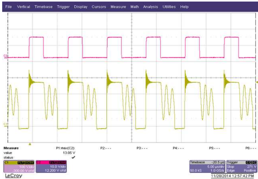
Figure 11. C1 = V_{SW} , C2 = V_{DRV} 115 V, 30 W
