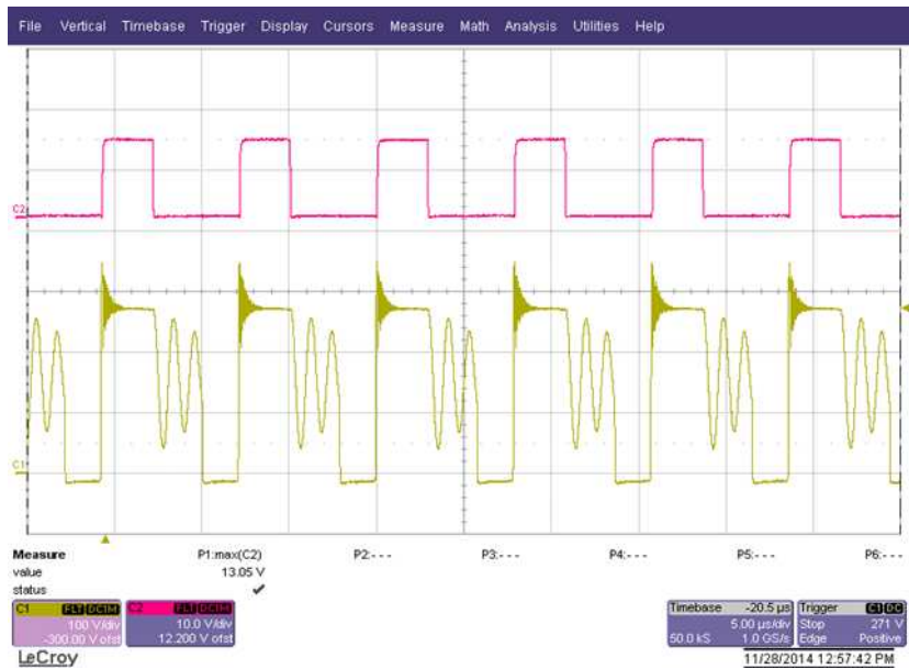
Figure 12. C1 = V_{SW} , C2 = V_{DRV} 230 V, 30 W
