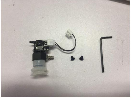
**Step 1:** Fix the suction cup to the front mounting block with the M3 screws.
