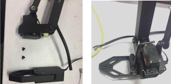
Step 2: Plug the wire of gripper
