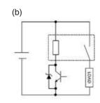
OMRON recommends coil driver circuit (b) and (c) for coil surge suppression. However the circuit (d) is not recommended because it may negatively affect the durability performance.
