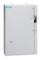
2-speed 3-phase motor starter Size 1 Two separate windings Constant or variable torque Solid-state overload relays Low SPD OLR range 0.75-3.4A High SPD OLR range 0.75-3.4A 110V 50HZ / 120V 60HZ coil Combination type 3Amp circuit breaker Encl NEMA type 4X 304 S-steel Water/dust tight noncorrosive
