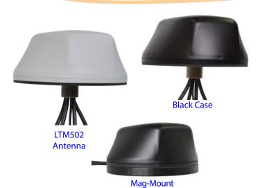
Mobile Mark's LTM502 Series Multiband Diversity/MIMO antenna contains five separate antennas, all in one compact antenna housing: two broadband LTE/Cellular antennas, two dual-band WiFi antennas, and one GPS antenna. The LTM502 differs from the LTM501 in that the broadband LTE/Cellular element covers all LTE frequencies worldwide, from 694-3700 MHz.
