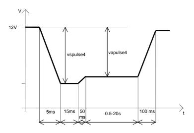
Test Pulse 5 (Load Dump) Ri = 0.5...4R (clamped to 40V during test)
