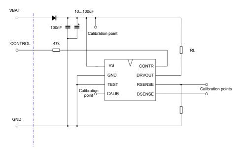
1.3.1. Electronic fuse schematic diagram
