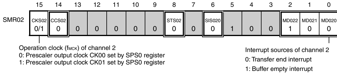
Figure 13-93. Example of Contents of Registers for Address Field Transmission of Simplified I 2 C (IIC10) (1/2)
