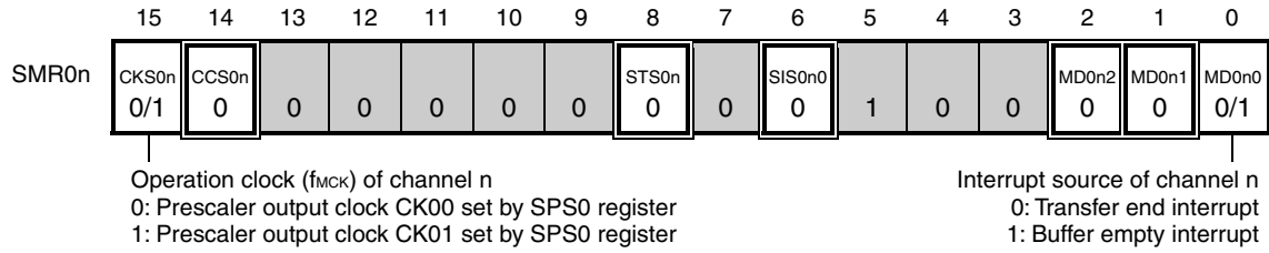
Figure 13-40. Example of Contents of Registers for Master Transmission/Reception of 3-Wire Serial I/O (CSI00 Note , CSI01 Note , CSI10) (1/2)
