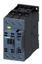
power contactor, AC-3e/AC-3, 51 A, 22 kW / 400 V, 3-pole, 175-280 V AC/DC, 50/60 Hz, with integrated varistor, auxiliary contacts: 1 NC, main circuit: screw terminal, control and auxiliary circuit: spring-loaded terminal, size: S2, F-PLC-IN
