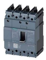
circuit breaker 3VA5 UL frame 125 breaking capacity class S 25kA @ 480V 4-pole, line protection TM210, FTFM, In=100A overload protection Ir=100A fixed short-circuit protection li=10 x In N conductor protection 100% without connection
