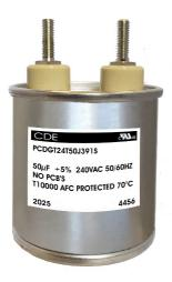
Type PCD capacitors are designed to meet the demands of AC filter applications rich in system total harmonic distortion (THD). This series has a patented dual protection system utilizing self healing metallized polypropylene and a mechanical pressure interrupter designed to operate while bus bar mounted or bottom stud mounted to ensure a safe open circuit mode in the event of overload or end of life.
