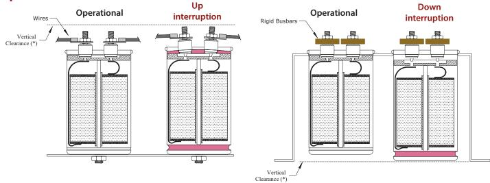
(\*) Vertical Clearance – Proper operation of the patented dual protection system requires that a minimum of 0.5" vertical clearance be carefully observed above the capacitor terminals if flexible connections are used or under the capacitor body if busbar mounted.
