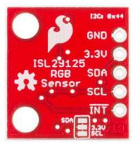
If you want to disable the on-board  $10k\Omega$  I²C pullup resistors – in case you want to use those built into your microcontroller or other external pull-ups – simply cut the two traces between the three pads on the backside of the board. If you decide you want the pull-ups later, you can always solder the pads back together.
