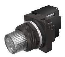
30mm BlackMax, Epoxy Coated Corrosion Resistant Complete Metal Unit Illuminated Indicator Light Full Voltage type, 24V AC/DC Incandescent Lamp, BA9s Glass Lens, Clear UL Listed, CSA Certified NEMA 1,3,3R,4,4X,12,13 & Automotive Standards
