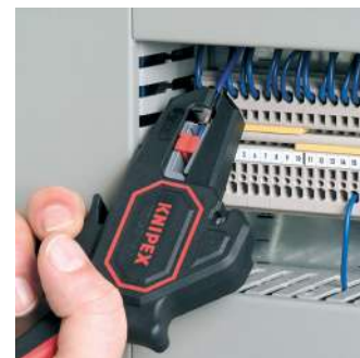
Stripping in confined areas
