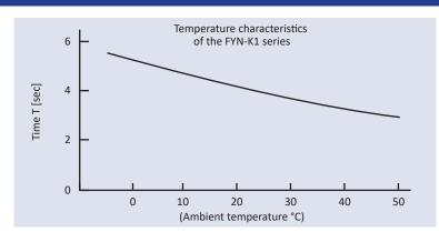
■ Damper characteristics vary according to the ambient temperature. In general, the damper characteristics become weaker as the temperature increases, and become stronger as the temperature decreases. This is because the viscosity of the oil inside the damper varies according to the temperature. When the temperature returns to normal, the damper characteristics will return to normal as well. The changes in the time it takes for the lid to close are shown in the graph to the left.
