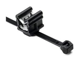
Outside Serrated Cable Tie & Edge Clip, 6.0" Long, EC20, 3-6 mm Panel, 50lb, PA66HS, Black, 500/pkg
