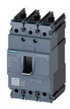
circuit breaker 3VA5 UL frame 125 breaking capacity class S 25kA @ 480V 3-pole, line protection TM210, FTFM, In=35A overload protection Ir=35A fixed short-circuit protection Ii=10 x In UL 489 SB (naval), 50° C without connection
