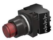
30mm BlackMax, Epoxy Coated Corrosion Resistant Complete Metal Unit PTT / Illuminated Pushbutton Full Voltage, 120V AC/DC Incandescent Lamp Extended Button Plastic Lens, Red 2 Position Momentary with 1 N.O. - 1 N.C. Heavy Duty Contacts, A600/P600 UL Listed, CSA Certified NEMA 1,3,3R,4,4X,12,13 & Automotive Standards
