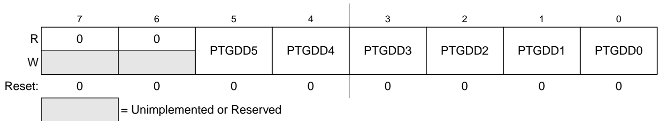
Figure 6-43. Port G Data Direction Register (PTGDD)
