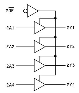
FIGURE 4. Logic diagram.
