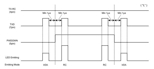
\*If TX-RC or TXD input pulse width is wider than 48µs, output LED emitting pulse will be turn off approximately 48µs.
