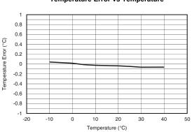
**Temperature Error vs Temperature**
