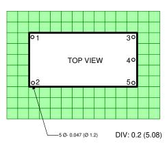
Dimensions: inch (mm) Case Tolerance: ± 0.02 (0.50) Pin Pitch Tolerance: ± 0.012 (0.30)
