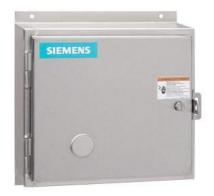
Non-reversing contactor, Size 1 3/4, Three phase full voltage, Contactor amp rating 40A, 3 wire (NO aux included), 110-120/220-240VAC 60Hz coil, Non-combination type, Encl NEMA type 4X 304 S-Steel, Water/dust tight noncorrosive, Extra-wide enclosure
