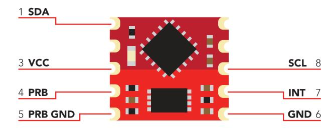
The pH OEM™ circuit requires two separate ground planes to operate properly. One ground plane is for the digital section of the device, the other is for the analog section.
