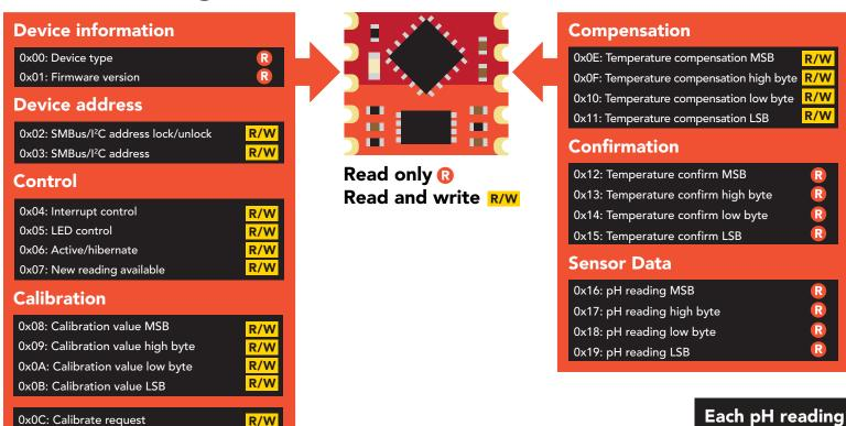
The default device address is **0x65** This address can be changed.
