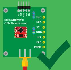
Do not solder wires to this device.
