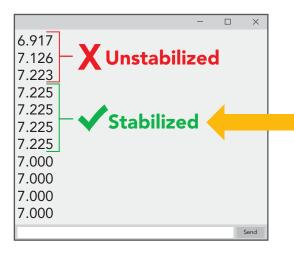
Once the readings have stabilized, calibrate to pH 7.
