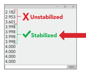
Once the readings have stabilized, calibrate to pH 4.
