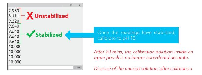
The pH OEM™ circuits default temperature compensation is set to 25° C. If the temperature of the calibration solution is +/- 2° C from 25° C, consider setting the temperature compensation first. Temperature changes of < 2° C are insignificant.
