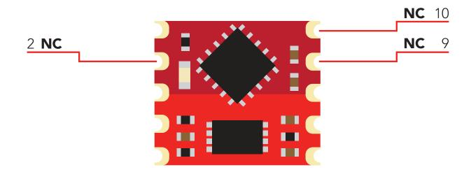
If the pH OEM™ circuit is going to be hand soldered, avoid using rosin core solder. Use as little flux as possible. Do not let liquid flux seep under the pH OEM™ circuit. After the pH OEM™ circuit has been soldered to the PCB all flux residue MUST be removed. Failure to do so will result in poor quality readings.
