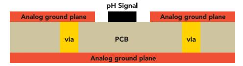
This cross section is an example of how the analog ground plane protects the pH signal. The analog ground should surround the pH signal, on both the top and bottom layers.
