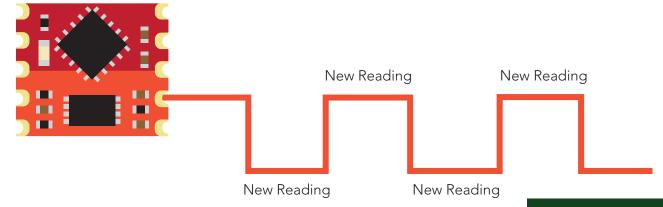
The pin will automatically invert its state each time a new reading is available. This setting has been specifically designed for a master device that can use an interrupt on change function.
