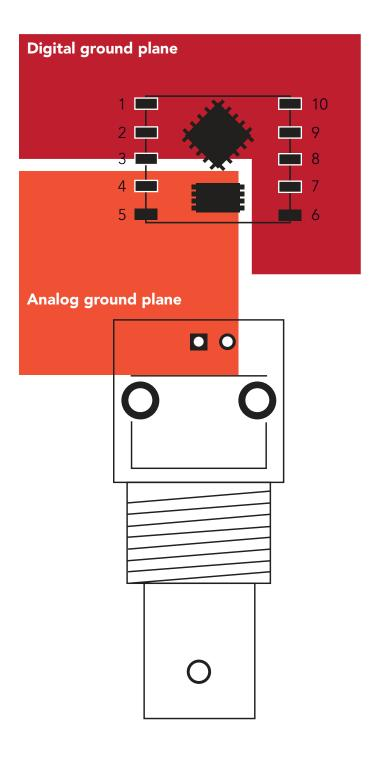
Using a 0.4mm trace width connect pin 4 (PRB) to pin 1 on the BNC/SMA. Keep this trace as short as possible. This trace is the pH signal path.
