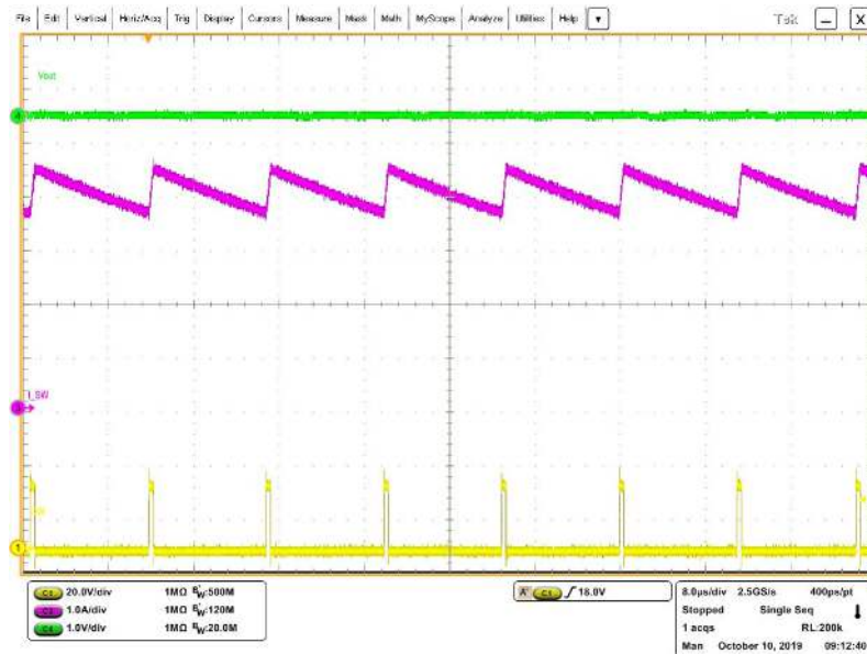
Figure 21. Over current procedure with persistent short circuit between V OUT and GND
