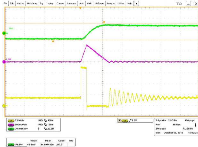
Figure 8. LCM operation with I_{SKIP} = 600 \text{ mA typ.} at zero load. L = 15 \mu\text{H} ; C_{OUT} = 40 \mu\text{F}
