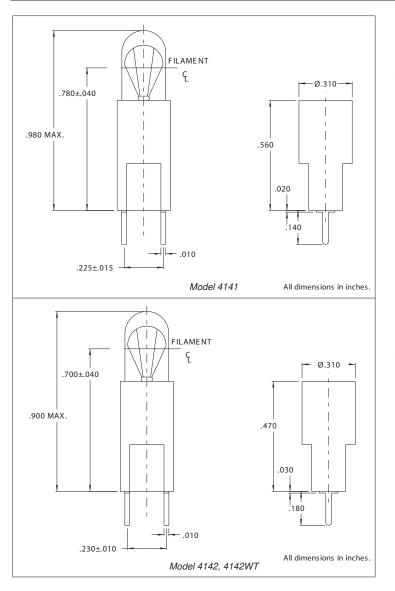
Mounting: Printed circuit Board Mounting pattern on page SP2. Terminals: Tinned brass Housing: White nylon Lamp: T-1 3/4 Wedge base Note: Lamps must be ordered separately.
