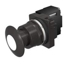
30mm BlackMax, Epoxy Coated Corrosion Resistant Complete Metal Unit Illuminated Push-Pull Operator Transformer type, 480V AC LED Lamp Mushroom Head Cap Small 1 3/4" (44.5 mm) Metal, Black with White Lens 3 Position Momentary UL Listed, CSA Certified NEMA 1,3,3R,4,4X,12,13 & Automotive Standards
