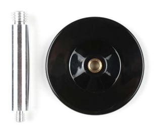
This is a very handy magnetic mount for survey grade GNSS/GPS antennas. Sturdy, compact, and surprisingly strong, this is a quick way of mounting your antenna to metal roofs, parapets, and other ferrous materials. The rod is threaded 5/8" 11-TPI (threads per inch) found on high-end surveying antennas and equipment. Additionally, the mount is tall enough to prevent kinking or collision between the TNC connector, cable, and the roof surface.
