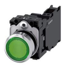
Illuminated pushbutton, 22 mm, round, metal, shiny, green, pushbutton, flat, momentary contact type, with holder, 1 NO+1 NC, LED module with integrated LED 24 V AC/DC, Spring-type terminal
