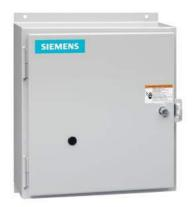
Mechanically held lighting contactor, Contactor amp rating 30Amp 0NC  $\_5NO$  poles, 440VAC 50HZ/480VAC 60HZ coil, Non-combination type, Enclosure NEMA type 12, Dust/drip proof for indoors
