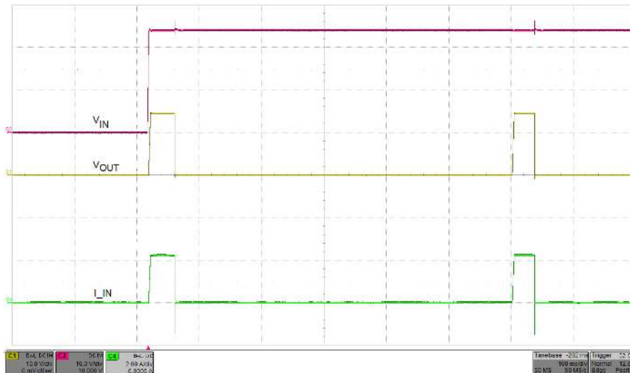
Figure 4. J5/J12 = 2-3 Position, Current Limit (2.23 A), Auto-Retry Mode
