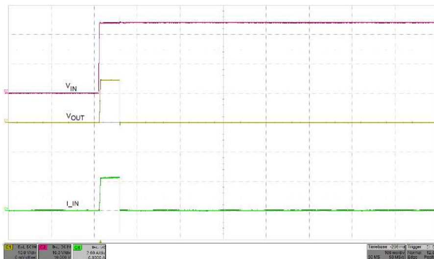
Figure 5. J5/J12 = 1-2 Position, Current Limit (2.23 A), Latch-Off Mode
