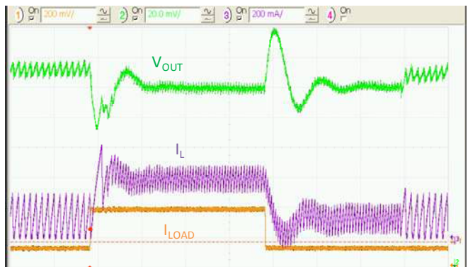
Figure 22. Load Transient 150mA to 400mA, V_{IN}=3.6V , t_{RISE}=t_{FALL}=100ns , 5 \mu s /div.
