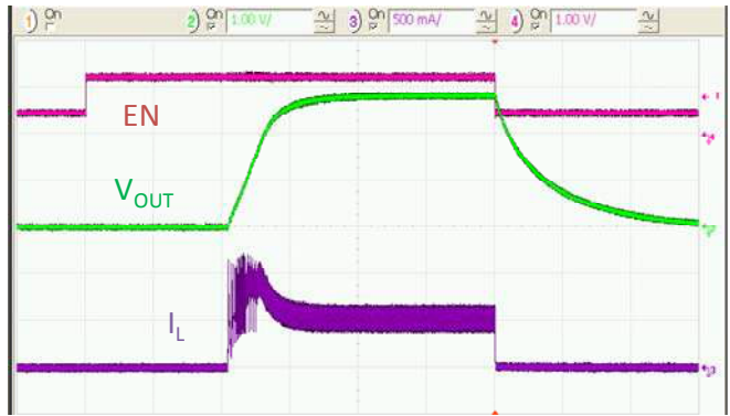
Figure 18. Startup and Shutdown through V_{EN} with 500mA Load, 50 \mu s /div.
