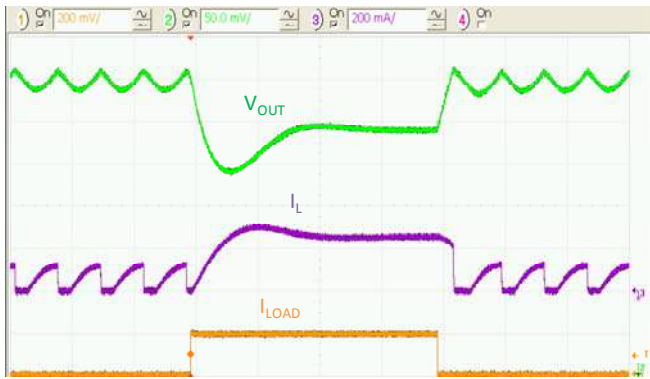
Figure 23. Load Transient 50mA to 250mA, V_{IN}=3V , t_{RISE}=t_{FALL}=100ns , 5\mu s/div .
