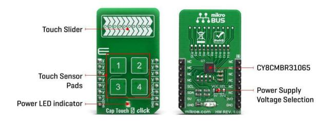
Advanced features, such as LED brightness control, proximity sensing, and system diagnostics, save development time. These controllers enable robust liquid-tolerant designs by eliminating false touches due to mist, water droplets, or streaming water. The CapSense controller locks up the user interface in firmware to prevent touch inputs in streaming water.
