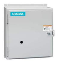
Non-reversing contactor, Size 2 1/2, Three phase full voltage, Contactor amp rating 60A, 3 wire (NO aux included), 24VAC 50-60Hz coil, Non-combination type, Enclosure NEMA type 12, Dust/drip proof for indoors, Extra-wide enclosure
